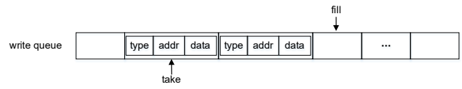
Fig. 3. The SPM-based batch processing for write requests
